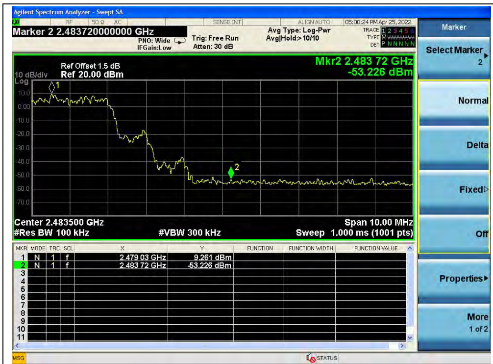
(Band edge with hopping on, Channel 78, 8-DPSK)
