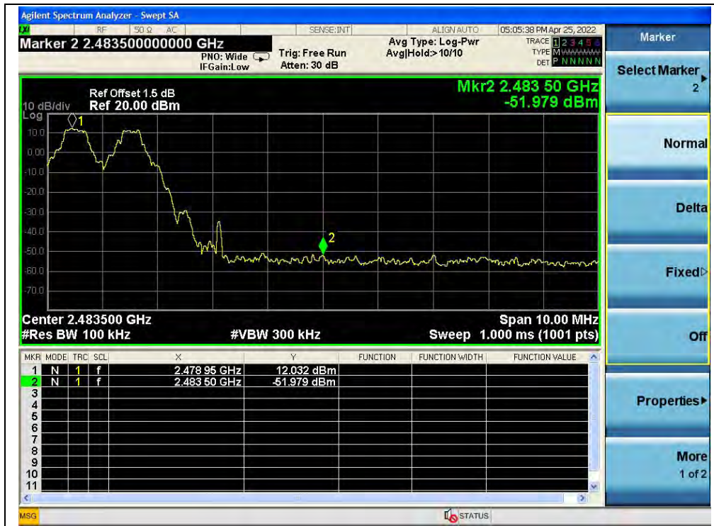
(Band edge with hopping on, Channel 78, GFSK)
