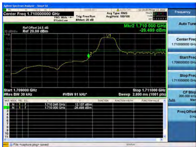
Band66 / 1.4MHz / High CH / QPSK / 1 RB
