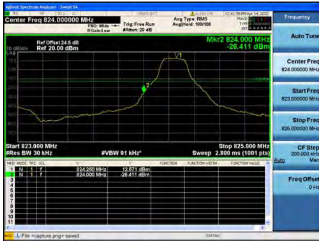
Band26 / 3MHz / High CH / QPSK / 1 RB
