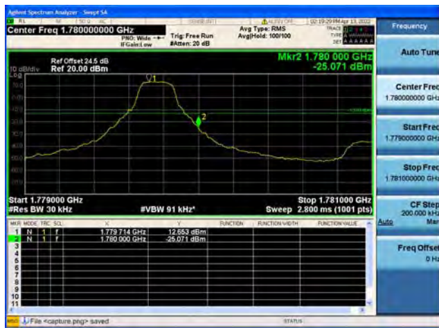
Band66 / 3MHz / High CH / QPSK / 1 RB
