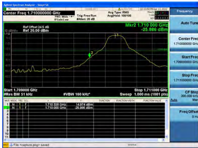
Band66 / 5MHz / High CH / QPSK / 1 RB
