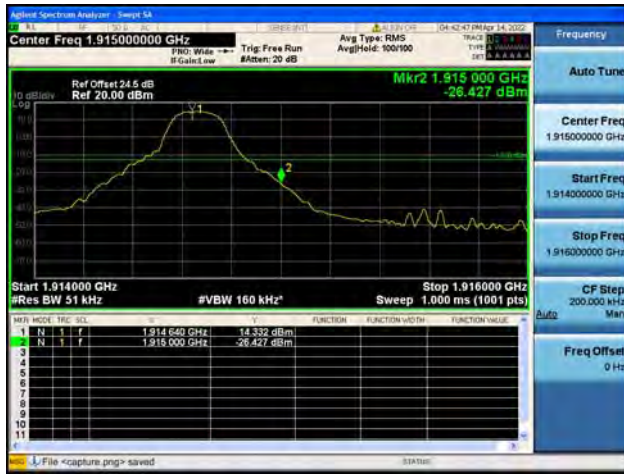
Band25 / 5MHz / High CH / QPSK / 1 RB
