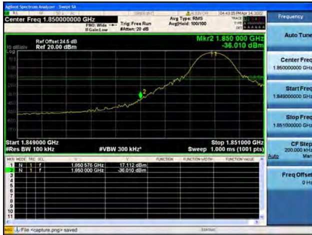
Band25 / 10MHz / High CH / QPSK / 1 RB
