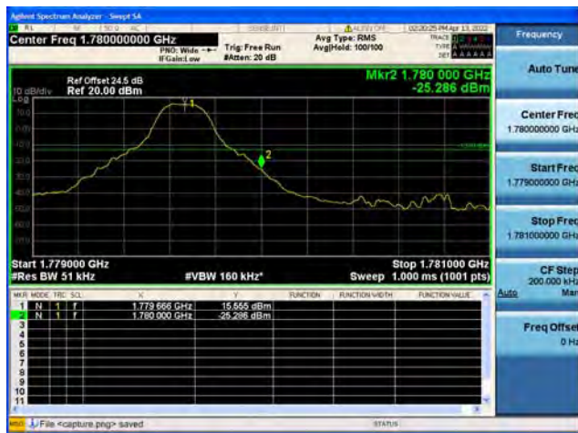
Band66 / 5MHz / High CH / QPSK / 1 RB
