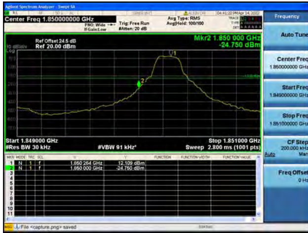
Band25 / 3MHz / High CH / QPSK / 1 RB
