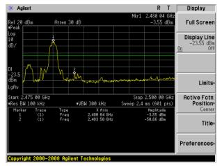
π /4-DQPSK: Band Edge-High Channel (Hopping Mode)
