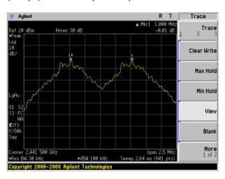
(2Mbps) Channel Separation plot on channel 39-40
