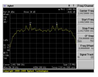
(1Mbps) Channel Separation plot on channel 77-78
