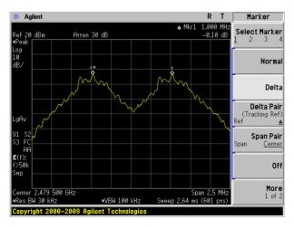
(2Mbps) Channel Separation plot on channel 77-78
