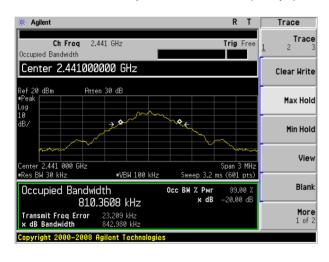
20dB Bandwidth plot on channel 39 (2Mbps)
