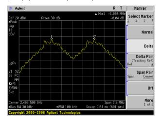
(2Mbps) Channel Separation plot on channel 00-01
