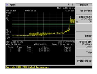
GFSK: Band Edge-High Channel (Hopping Mode)
