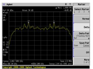
(1Mbps) Channel Separation plot on channel 39-40
