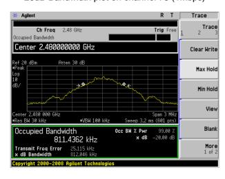
20dB Bandwidth plot on channel 78 (2Mbps)
