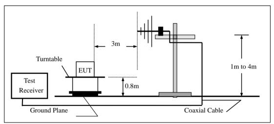
(c) For radiated emissions above 1000MHz
