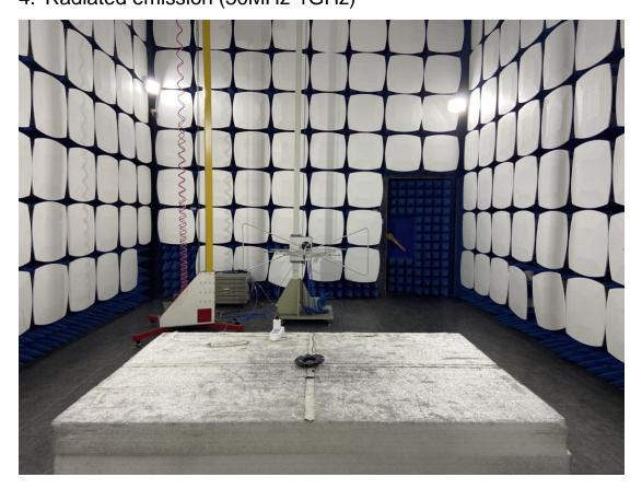
3. Radiated emission (9KHz-30MHz)
