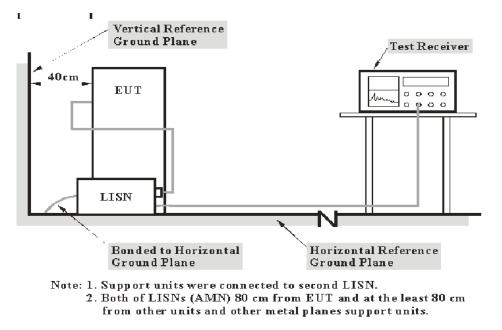
The setup of EUT is according with per ANSI C63.10-2013 measurement procedure. The specification used was with the FCC Part 15.207 limits.
