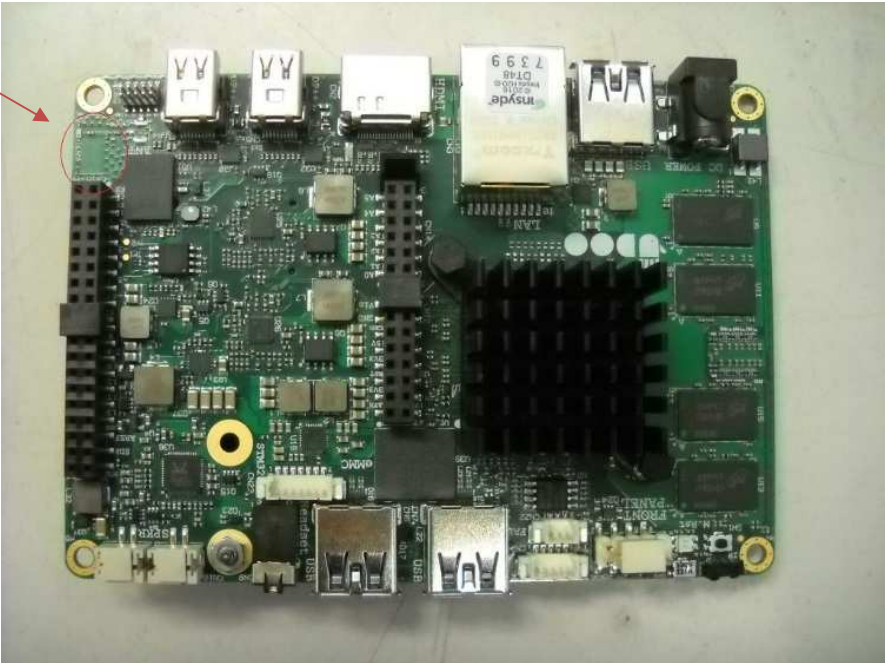
Figure 3.6-1: The Antenna is located on the PCB of EUT and not user accessible.
