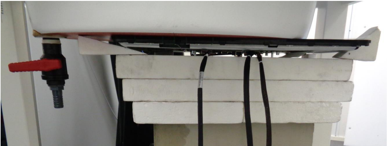
A2. Front side of the DUT against the phantom, 0mm separation distance
