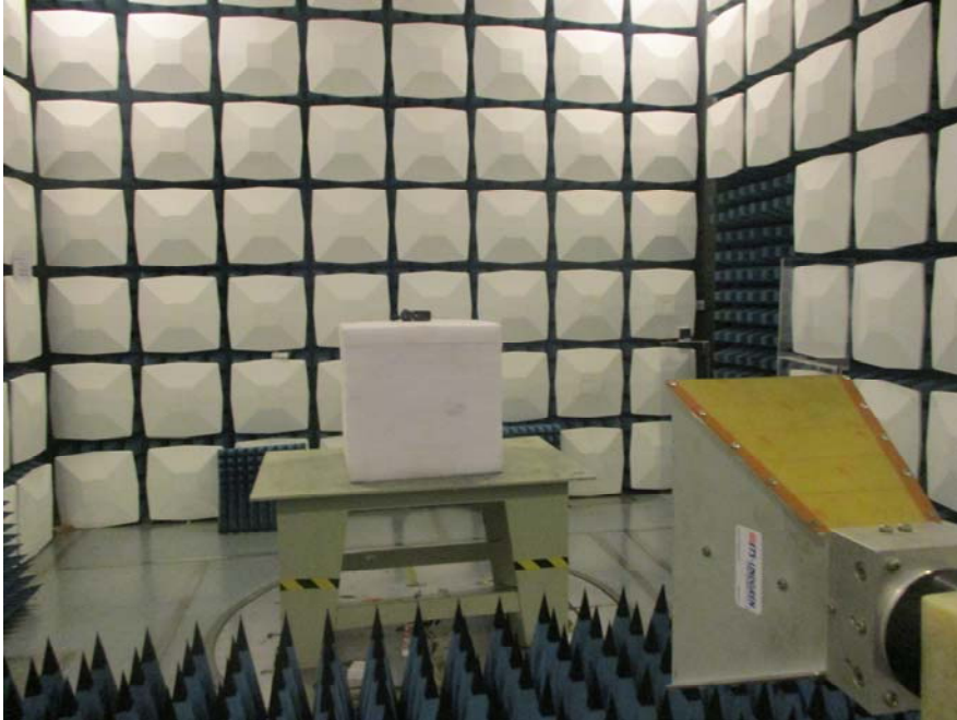
Radiated Emission View (Above 1GHz)
