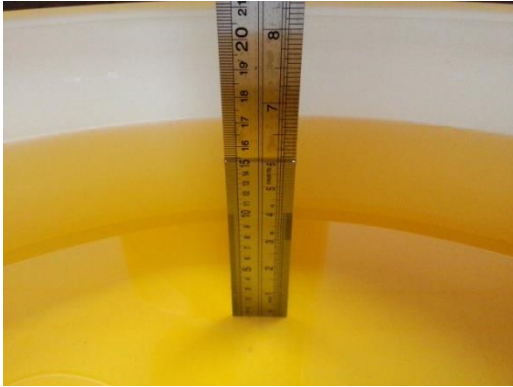
Photo 1: Tissue Simulant Liquid for Head 2300-2500
