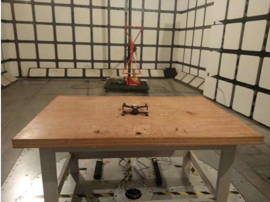
Radiated Emissions View (Below 1 GHz)
