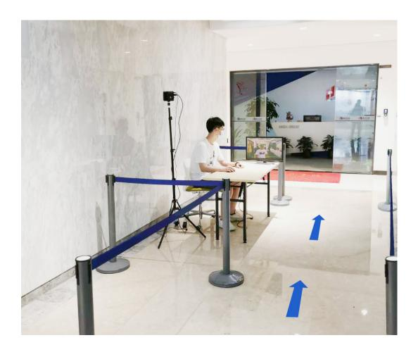
The distance between the detector and the object to be measured should be within 1-4m. As shown in the above figure, place the detector at an angle of 45 with the corridor, and ensure that the object to be measured can stay within the green box of the video for 1-3 seconds.
