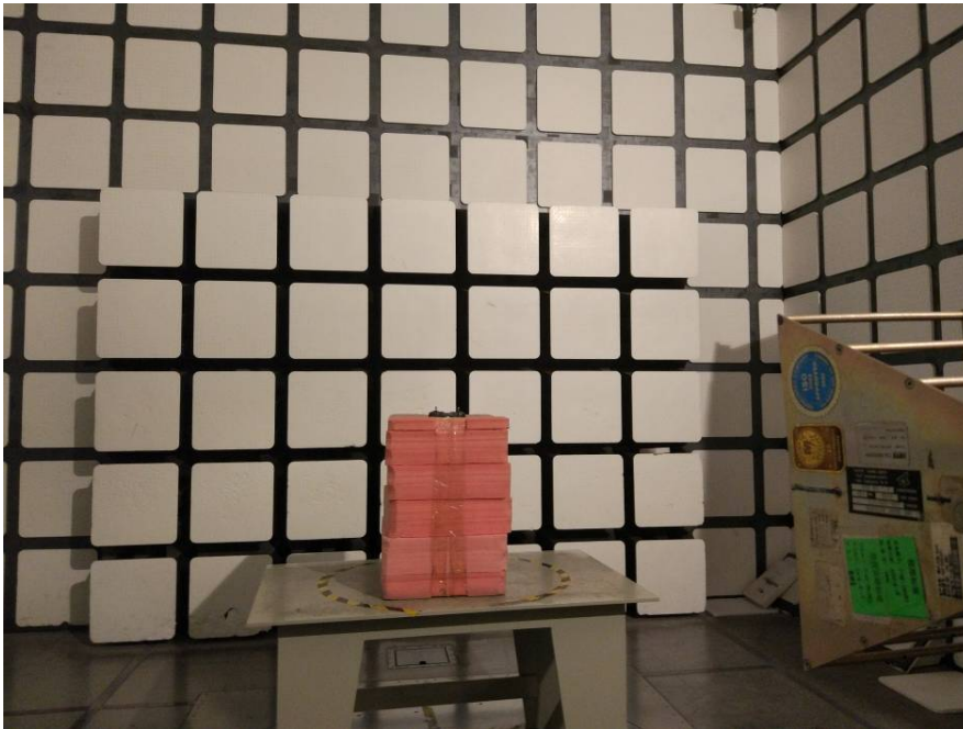
Radiated Emissions View (Above 1 GHz)
