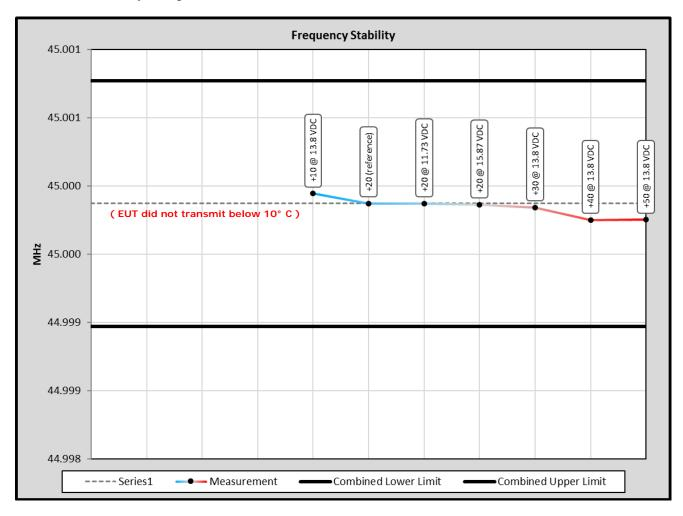
**Note:** The EUT stops operating at temperatures below 10° C. An FCC Inquiry was filed to address this failure to operate, and the FCC instructed that this was acceptable. The EUT, in no case, violates the frequency deviation limit of 20 ppm for this band.
