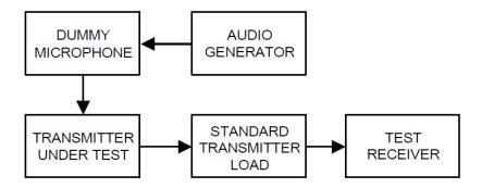
Test Data: Wideband - Modulation Limiting
