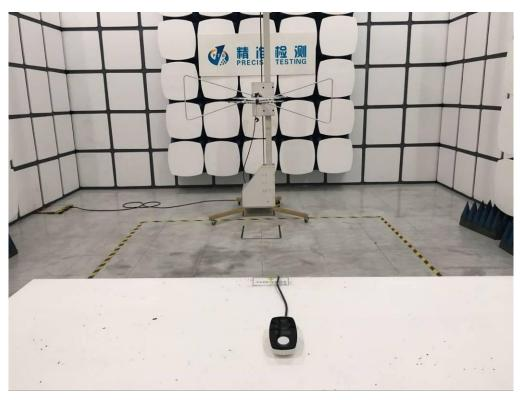
FCC RADIATED EMISSION TEST SETUP ABOVE 1GHZ
