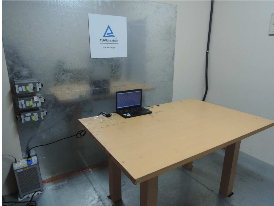
Photograph 6: Set-up for for Mains Conducted testing Front
