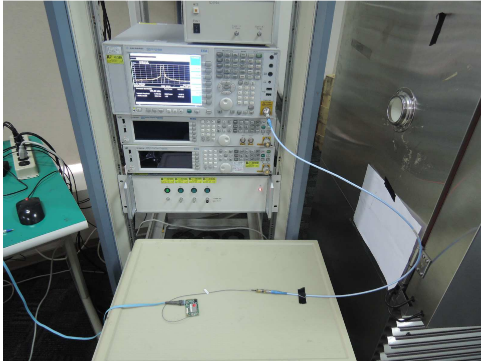
Photograph 5: Set-up for for Mains Conducted testing Back
