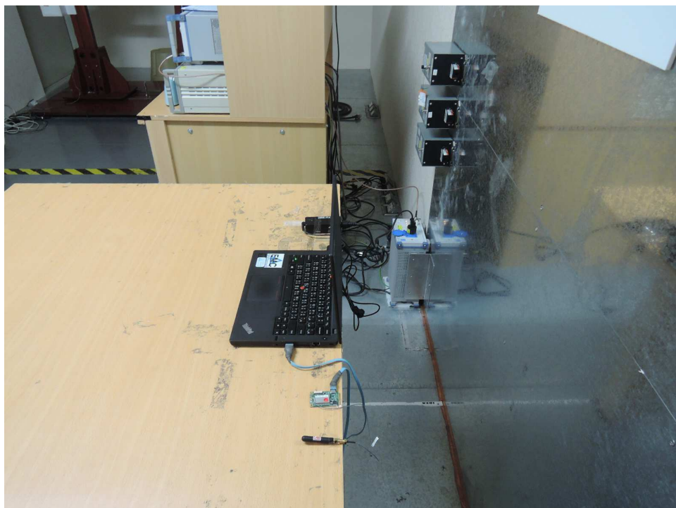
Photograph 5: Set-up for for Mains Conducted testing Back
