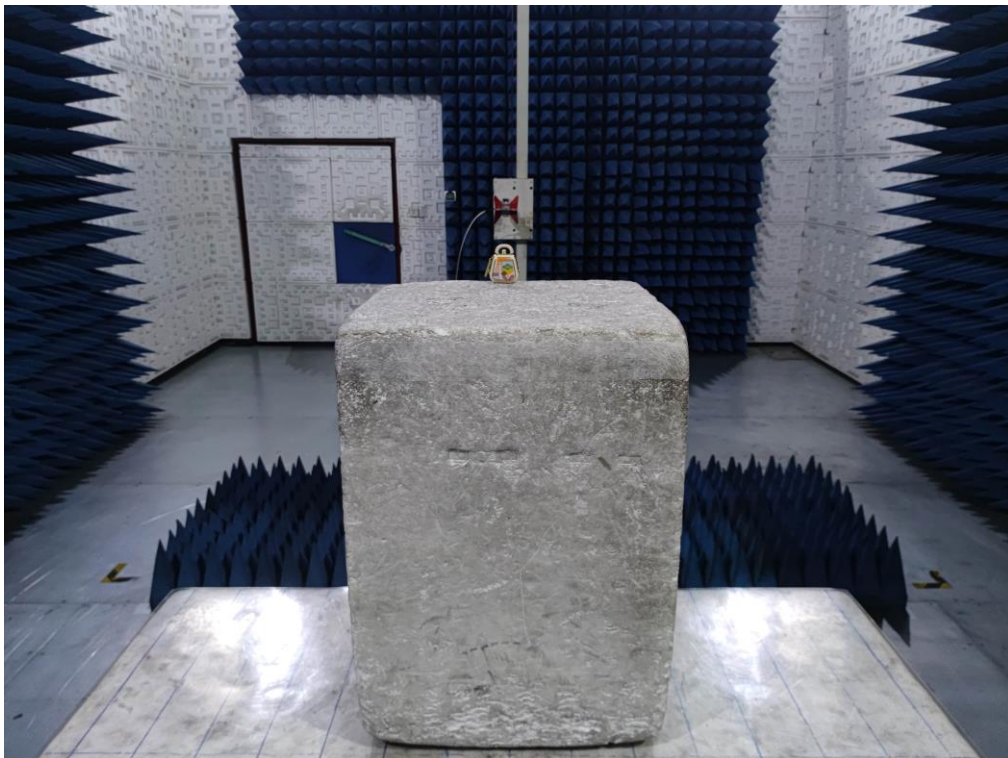
RADIATED EMISSION TEST SETUP ABOVE 1GHz
