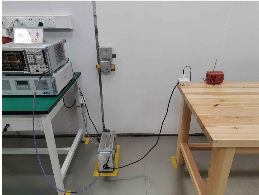
Conducted Emissions Test Setup
