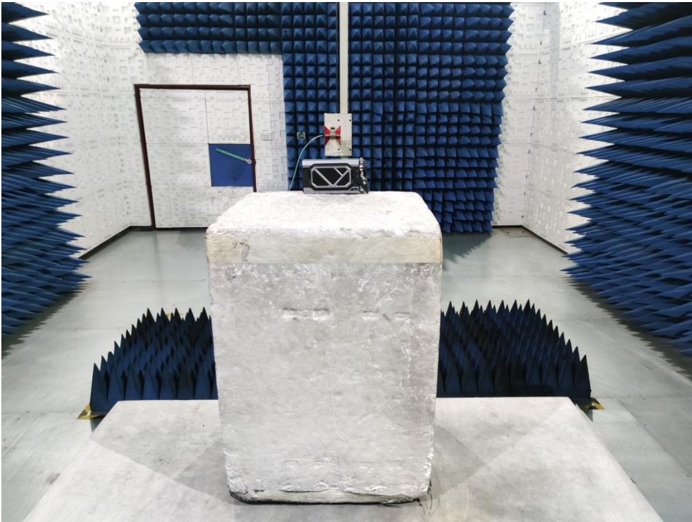
RADIATED EMISSION TEST SETUP ABOVE 1GHz
