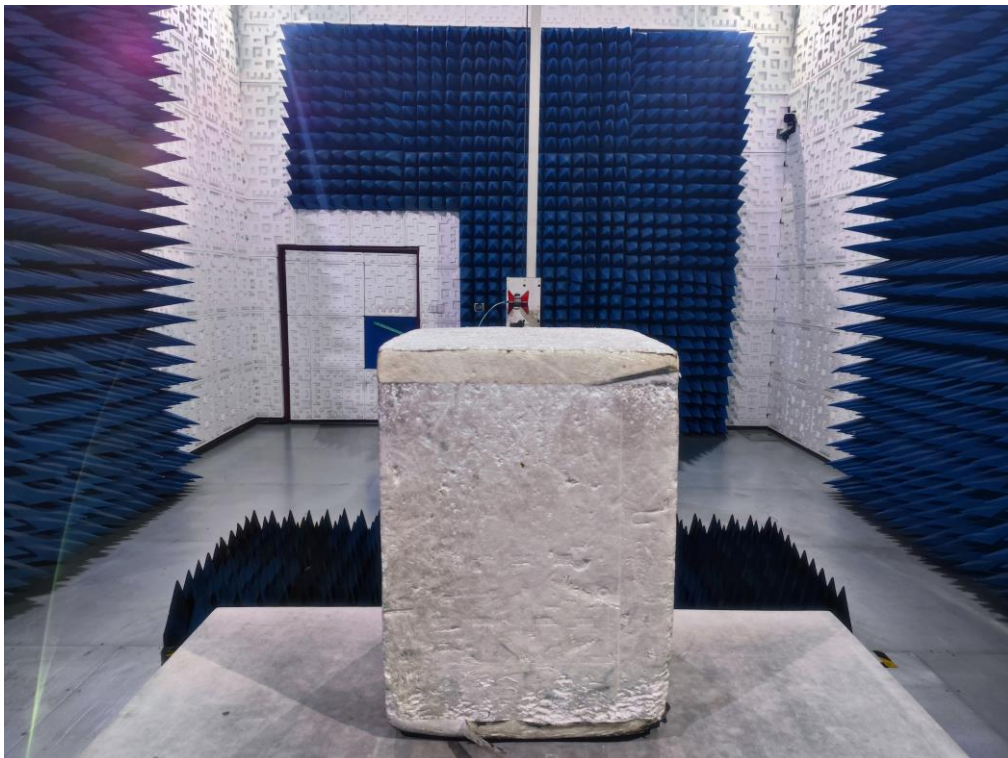
RADIATED EMISSION TEST SETUP ABOVE 1GHZ
