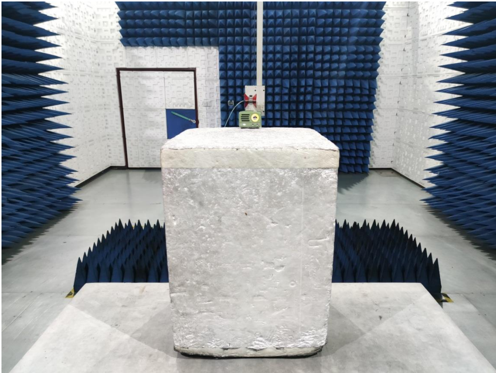
RADIATED EMISSION TEST SETUP ABOVE 1GHZ
