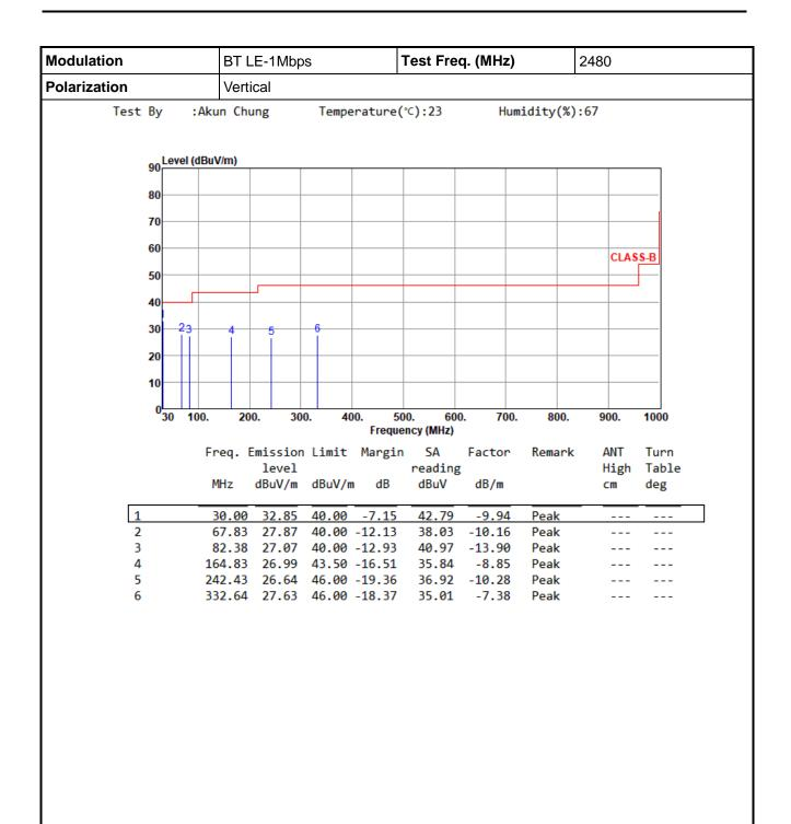
Note 1: Emission Level (dBuV/m) = SA Reading (dBuV) + Factor\* (dB/m)
