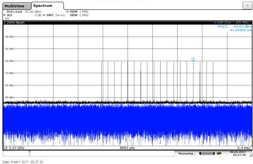
Channel Loading was approximately 17% - Data traffic was generated with the client device downloading data file from the server.
