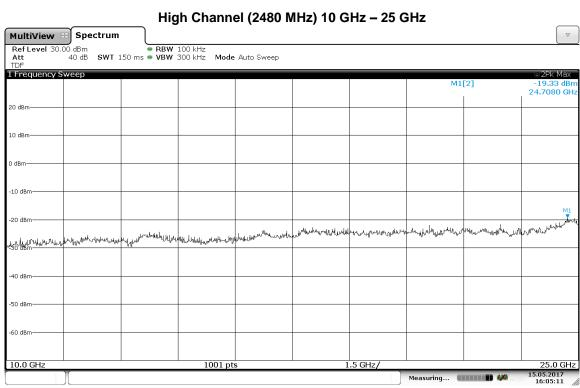
Note: Band edge test was performed on pi/4 DPSK modulation and DH5 data rate which recorded worst case 20 dB BW.
