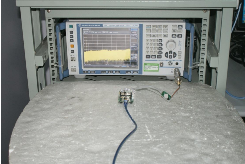
Photograph 2: Set-up for Spurious Emissions (9kHz-30MHz)
