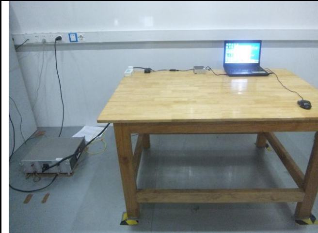
Conducted Emissions Test Setup Front View
