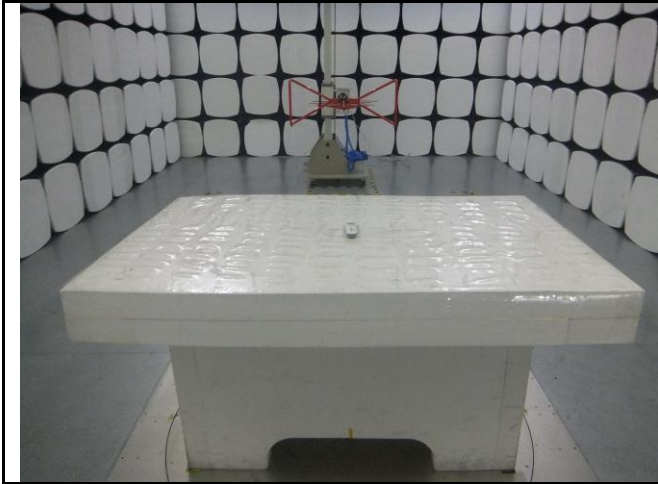
Radiated Emissions Test Setup Below 1GHz
