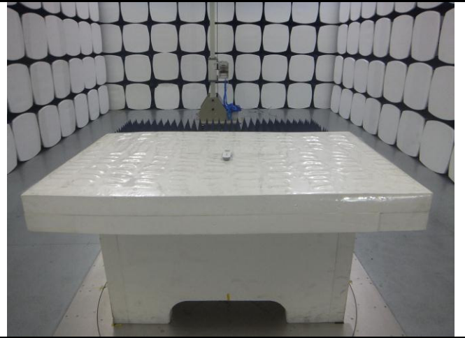
Radiated Emissions Test Setup Above 1GHz
