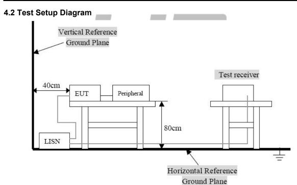
Remark: 1. The setup of EUT is according with per ANSI C63.10:2013 measurement procedure. The specification used was with the FCC 15.207 limits.
