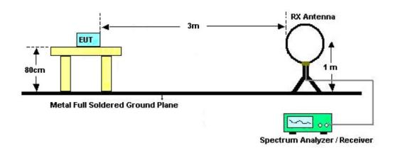
For radiated emission from 30MHz to1GHz
