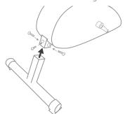
2. Use the screws to attach the Front Leg to the Cycle Case.
