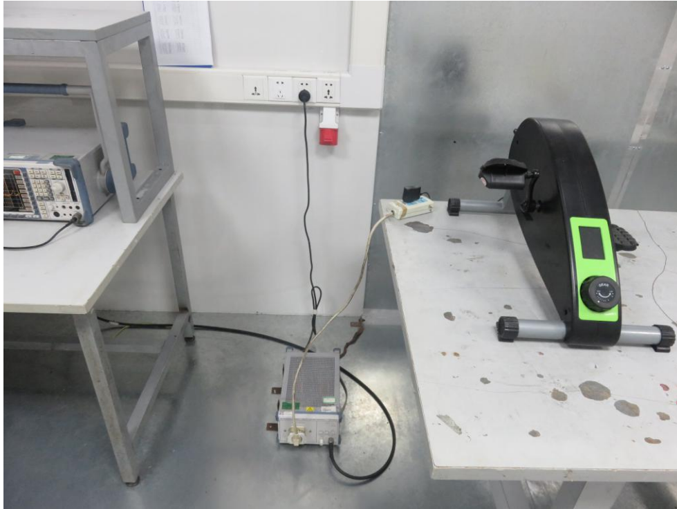
Photo of Conducted Emission Test
