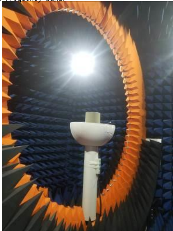
Fig. 4 Satimo anechoic chamber test system
