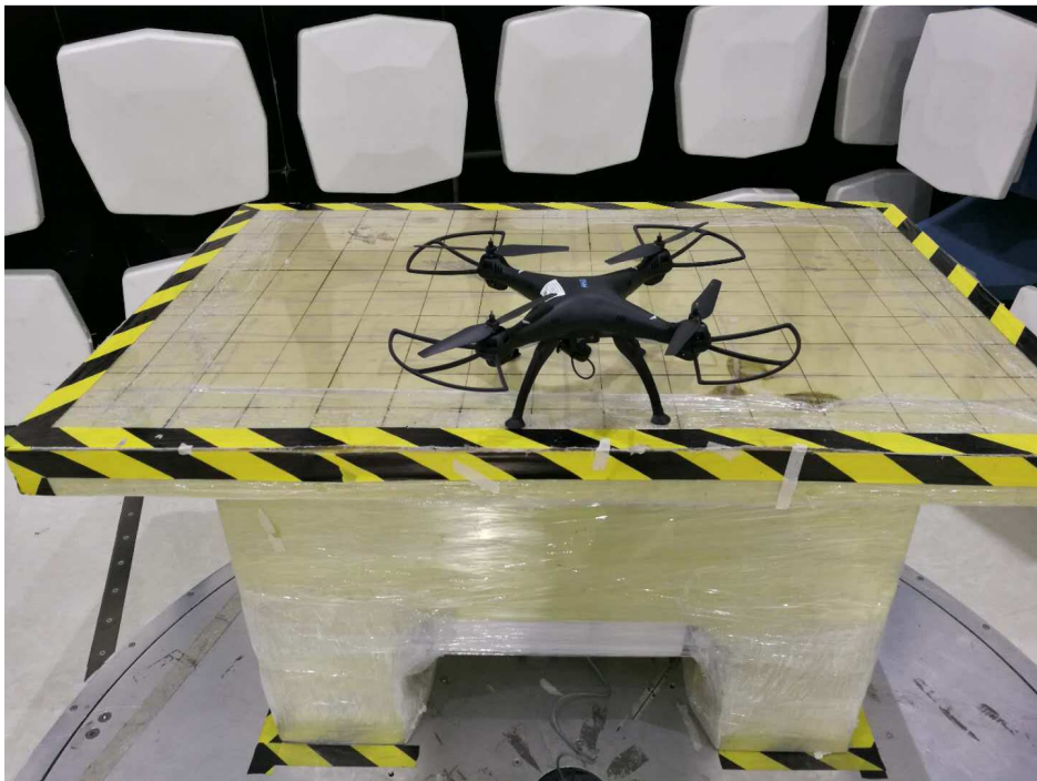
Up to 1GHz (Placed at the centre of the turntable)
