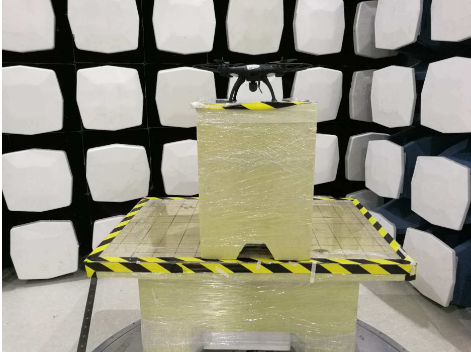
Above 1GHz (Placed at the centre of the turntable)
