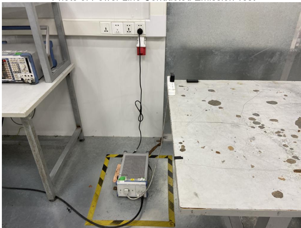
FCC ID: 2ALU5G102RX Photo of Power Line Conducted Emission Test
