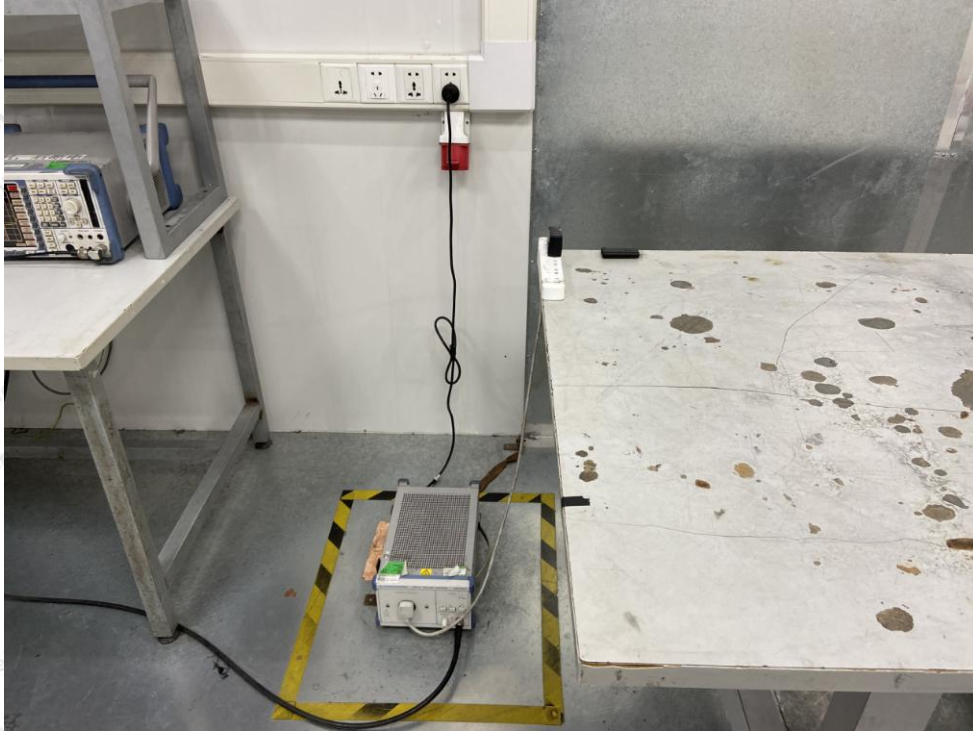
Photo of Power Line Conducted Emission Test
