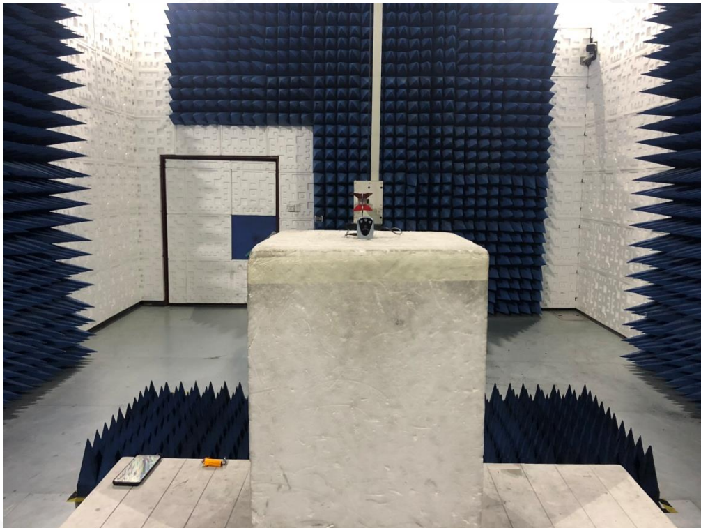
RADIATED EMISSION TEST SETUP ABOVE 1G
