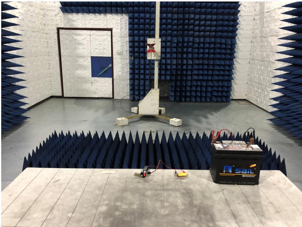
RADIATED EMISSION TEST SETUP ABOVE 1G
