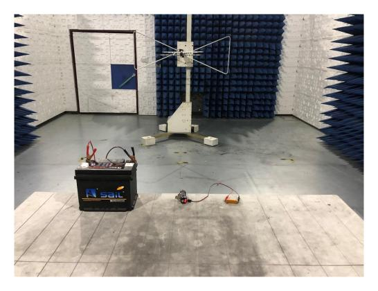
RADIATED EMISSION TEST SETUP ABOVE 1GHZ
