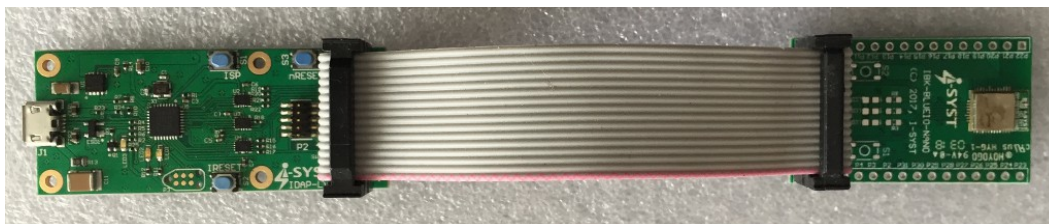
Fig. 5: IDAP-Link JTag with IBK-BLUEIO-NANO for development with the IMM-NRF52832-NANO module
