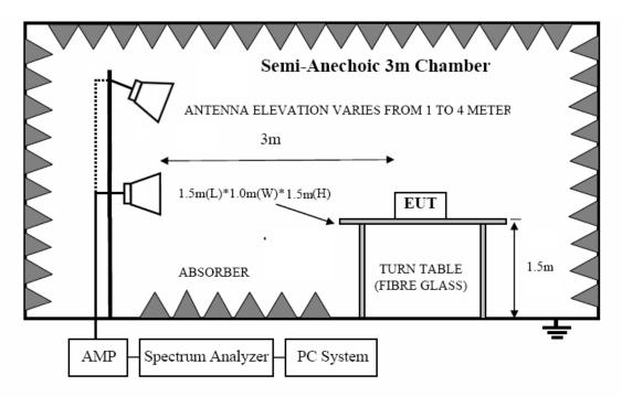
Note: For harmonic emissions test a appropriate high pass filter was inserted in the input port of AMP
