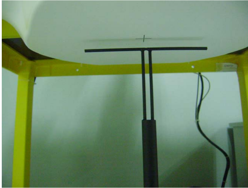
Setup Photo of Dipole Antenna
