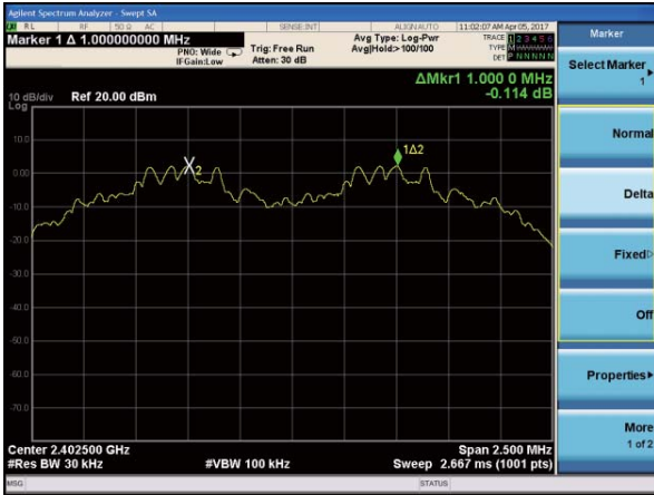
(3Mbps) Channel Separation plot on channel 39-40
