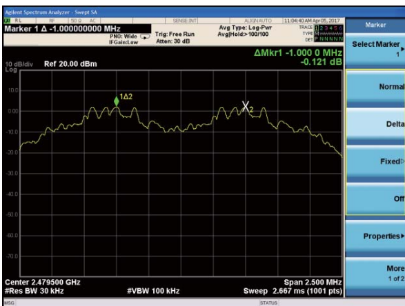
(3Mbps) Channel Separation plot on channel 77-78
