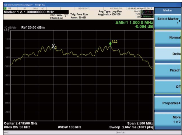
(2Mbps) Channel Separation plot on channel 77-78
