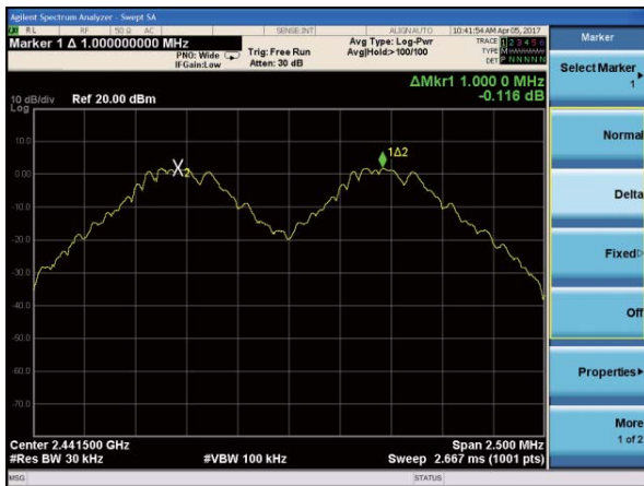
(1Mbps) Channel Separation plot on channel 39-40
