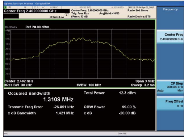
20dB Bandwidth plot on channel 39 (2Mbps)
