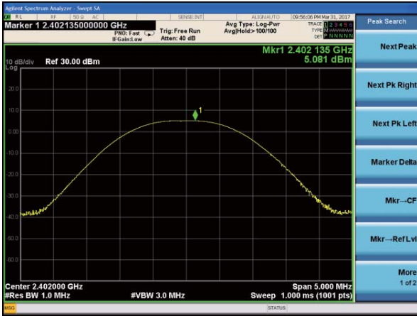
Peak output Power plot on channel 39 (1Mbps)
