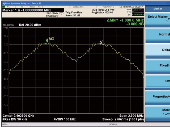
(1Mbps) Channel Separation plot on channel 39-40
