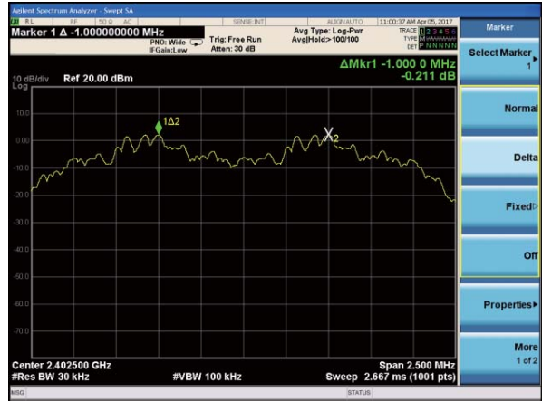
(2Mbps) Channel Separation plot on channel 39-40
