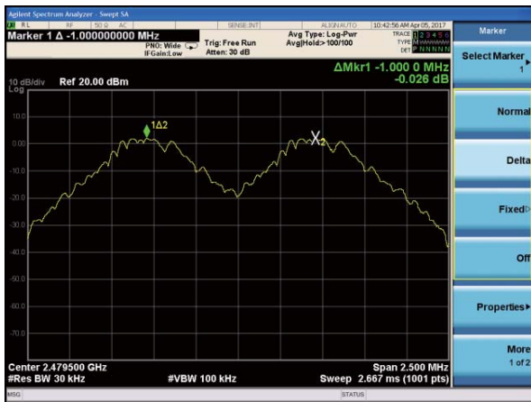
(1Mbps) Channel Separation plot on channel 77-78
