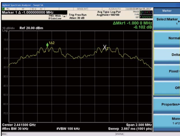
(3Mbps) Channel Separation plot on channel 39-40
