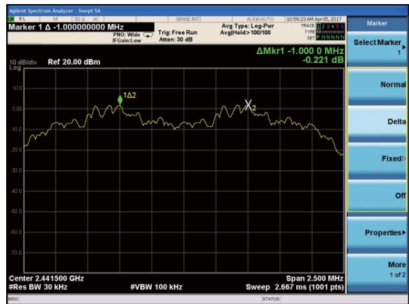
(2Mbps) Channel Separation plot on channel 39-40
