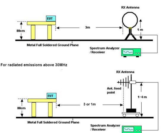
Above 10 GHz shall be extrapolated to the specified distance using an extrapolation factor of 20 dB/decade from 3m to 1m.
