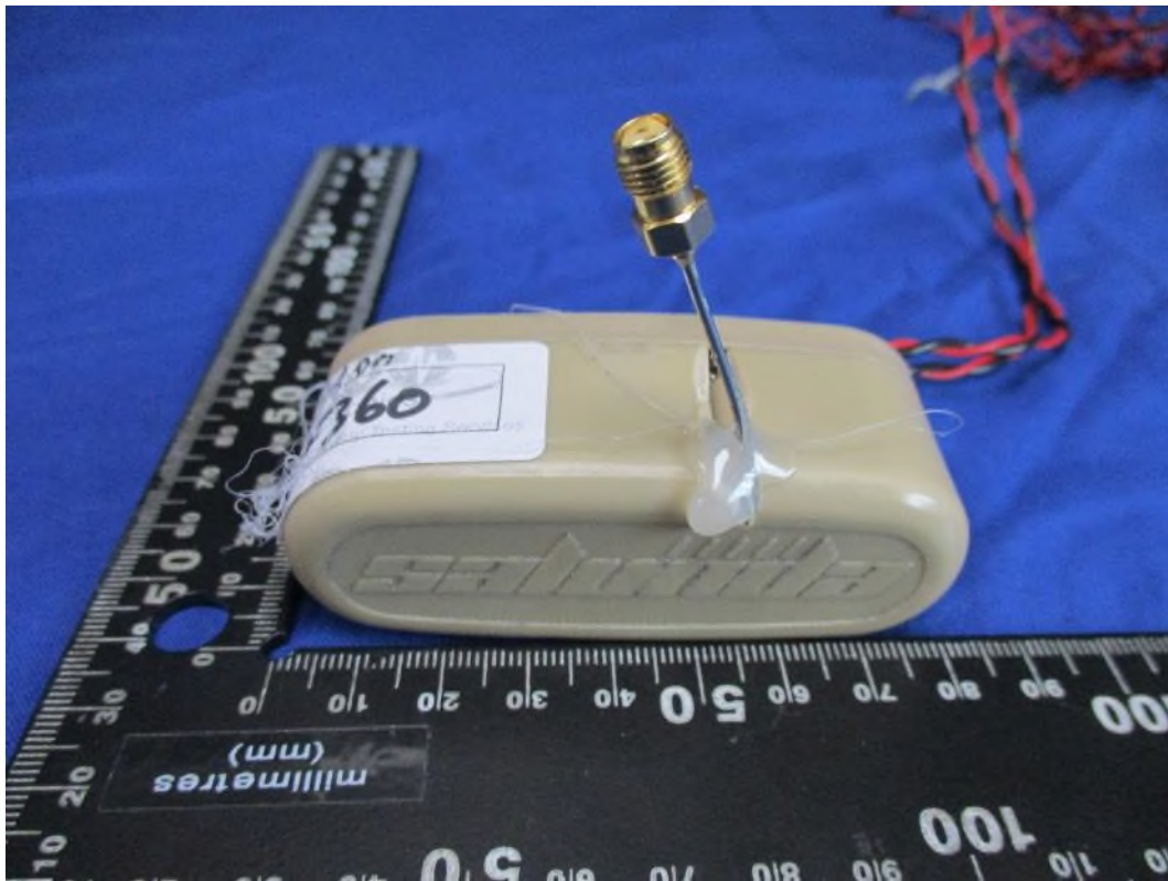
Conducted sample with temporary antenna port
