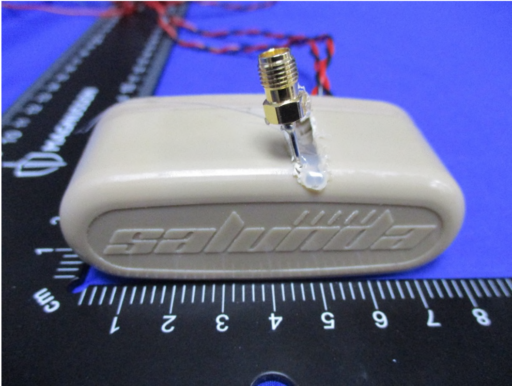
Conducted sample with temporary antenna port
