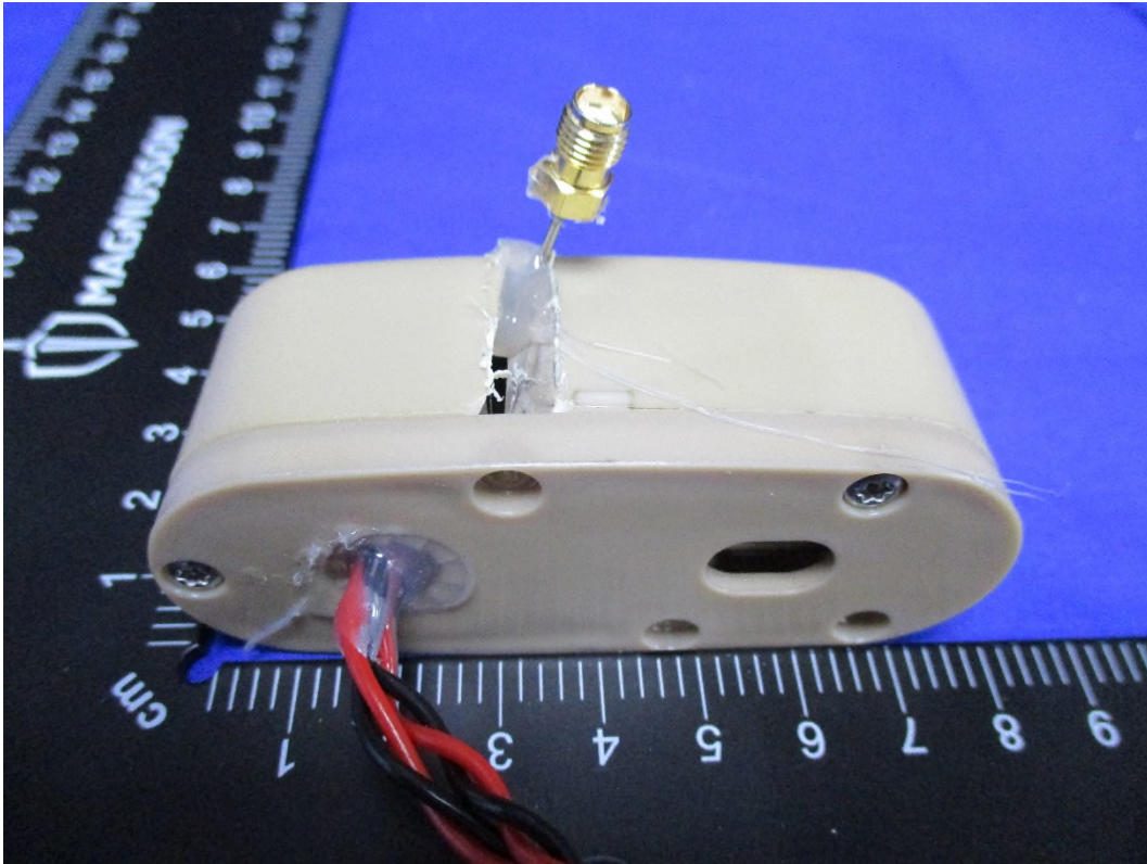
Conducted sample with temporary antenna port and DC cables fitted
