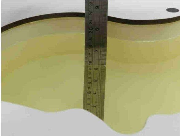
Fig 10.1 Photo of Liquid Height for Head SAR
