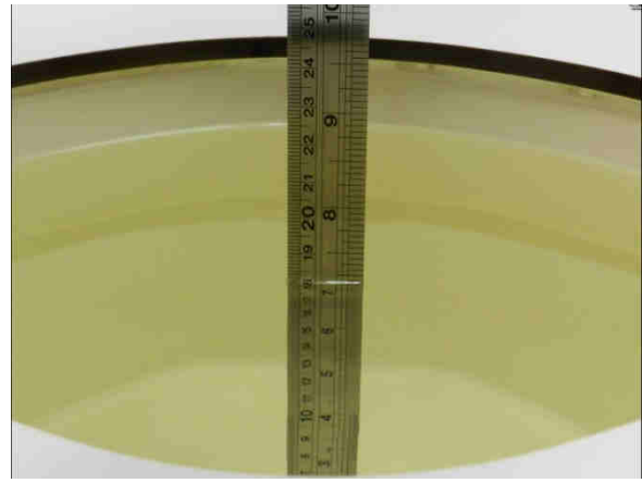
Fig 10.2 Photo of Liquid Height for Body SAR
