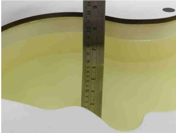
Fig 10.1 Photo of Liquid Height for Head SAR
