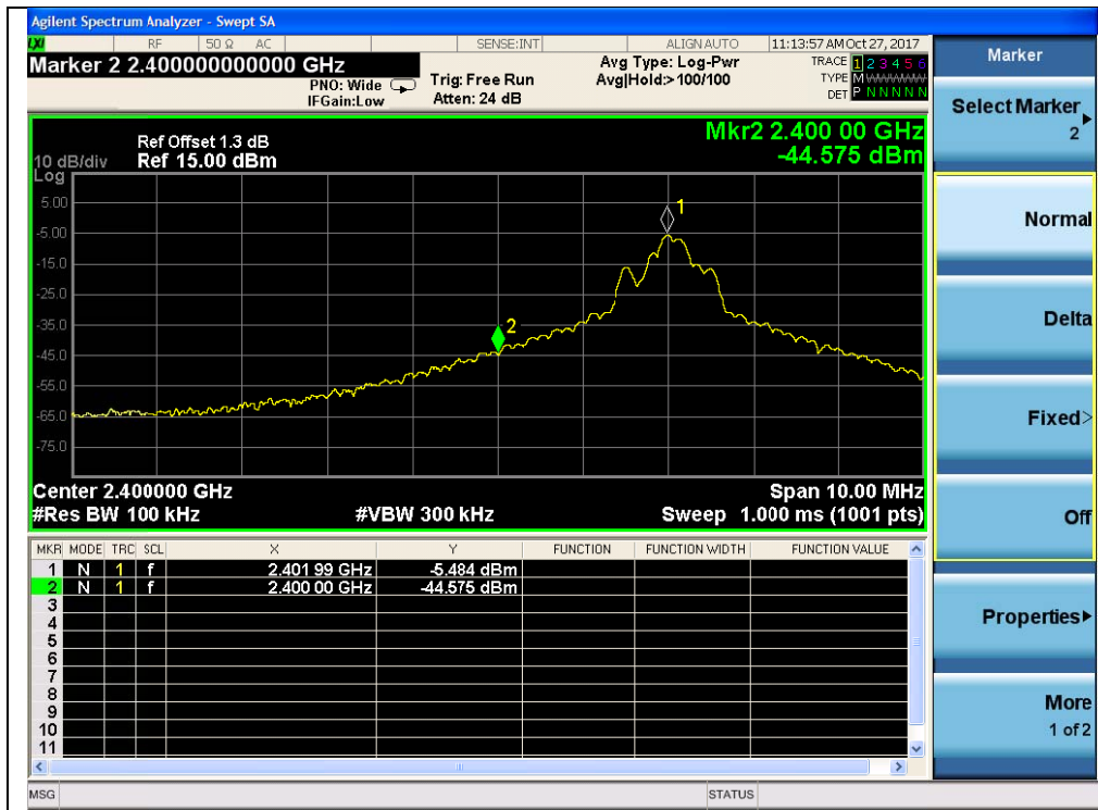
(Channel = 0, Band edge @ \pi/4 -DQPSK)
