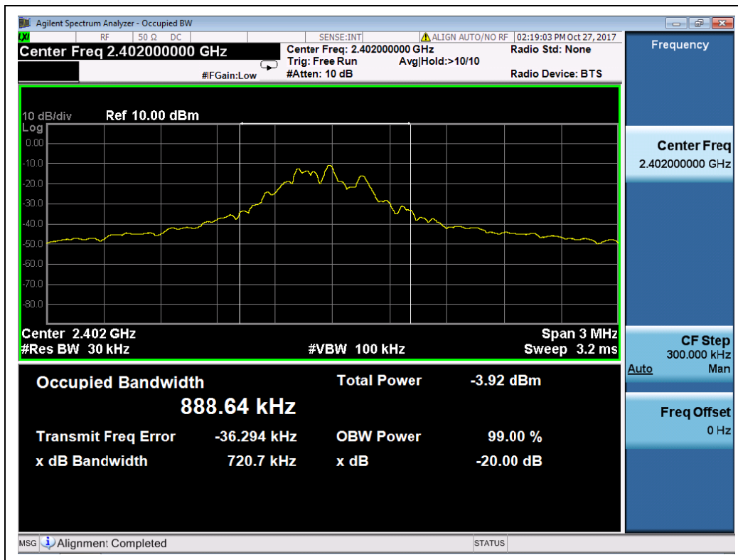
(Plot A: Channel = 2402 @ GFSK)
