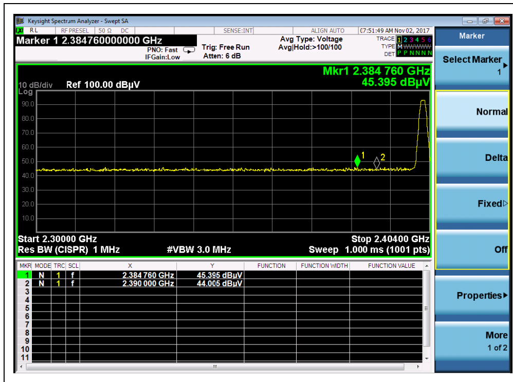
(Plot C1: Channel = 0 PEAK @ \pi/4 -DQPSK)
