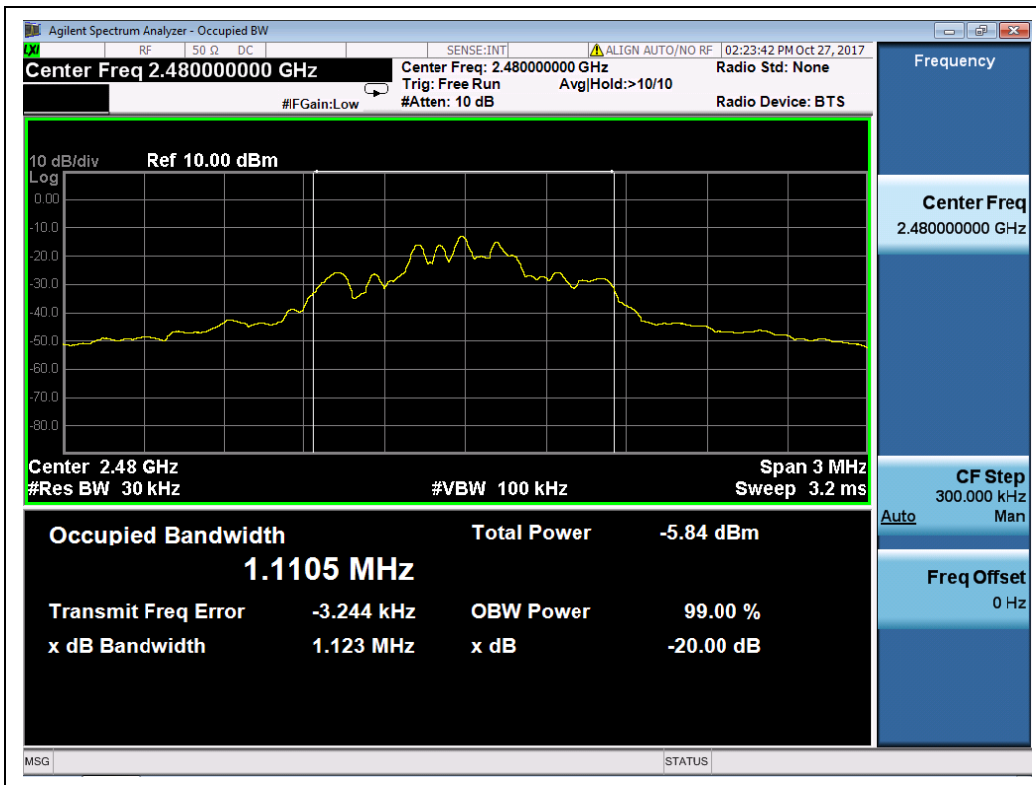
(Plot F: Channel = 2480 @ \pi/4 -DQPSK)
