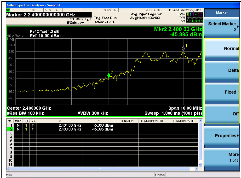
(Channel = 0, Band edge with hopping on @ 8-DPSK)
