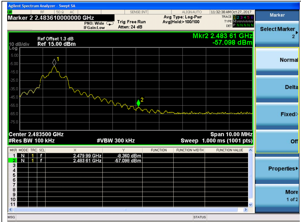
(Plot I.1: Channel = 78, Band edge @ 8-DPSK)
