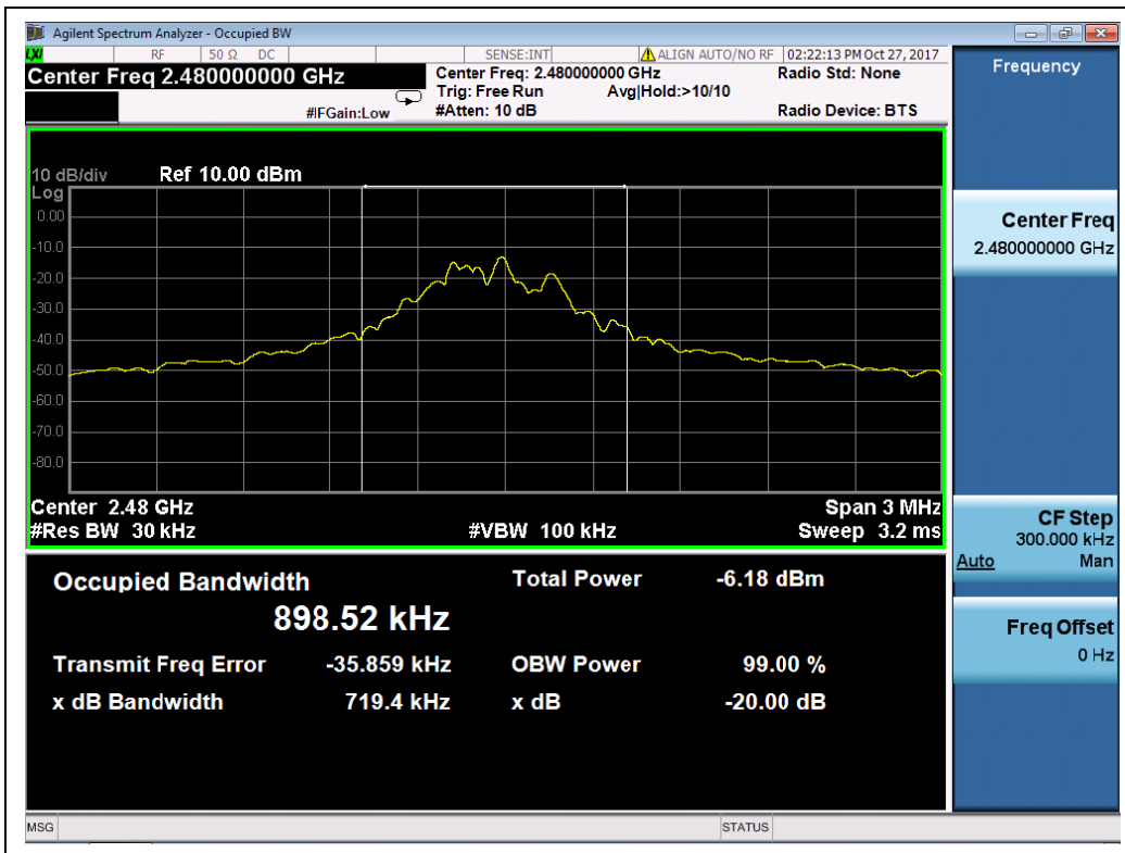
(Plot C: Channel = 2480 @ GFSK)
