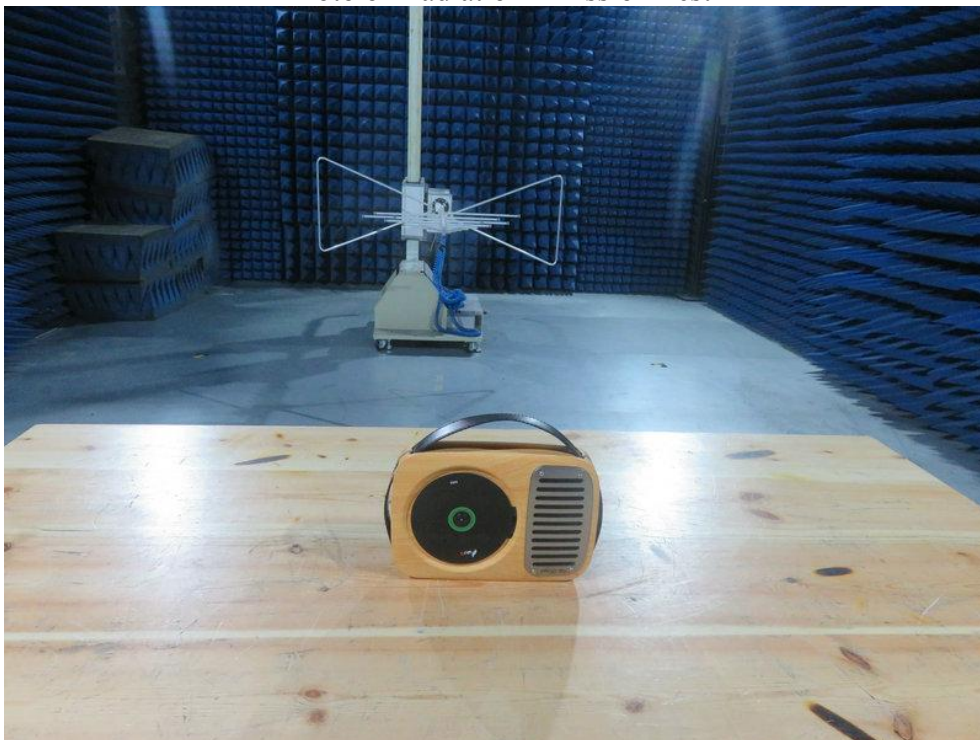
Photo of Radiation Emission Test
