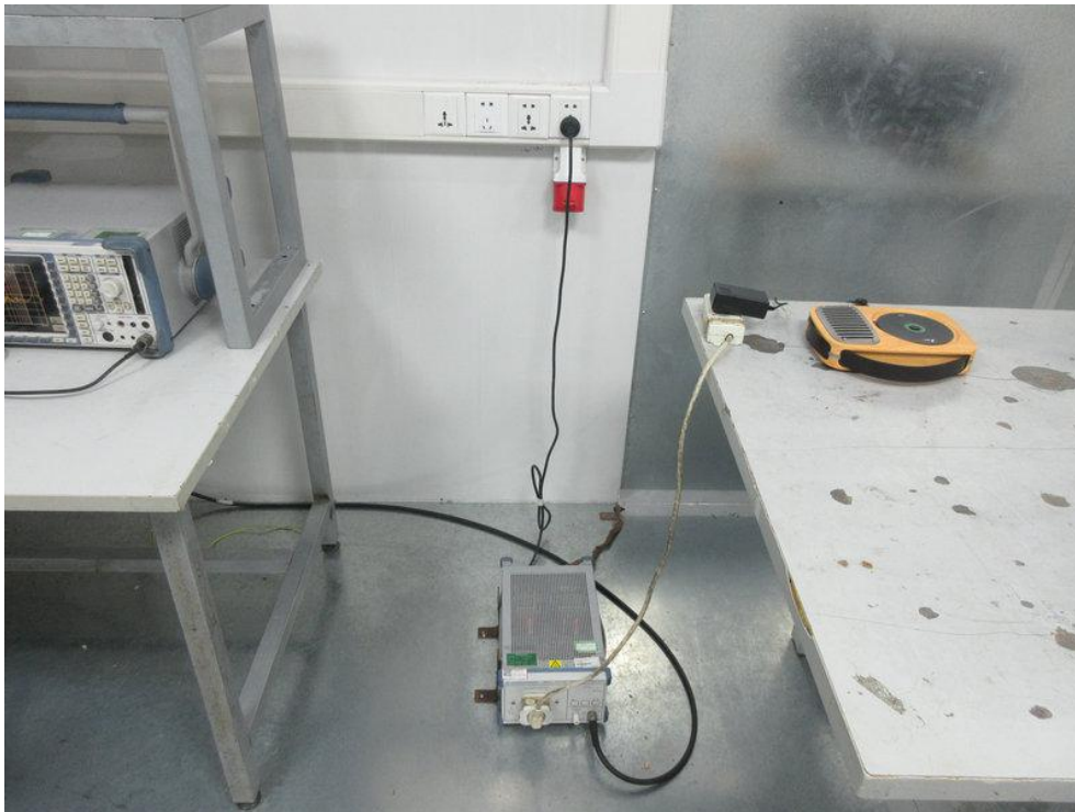
Photo of Conducted Emission Measurement
