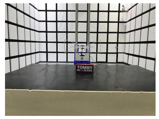
Spurious radiated emissions for transmitter and receiver:
